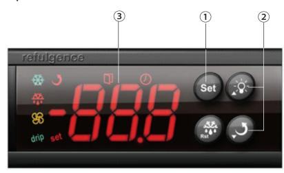
Range of temperature setting Refrigerated cabinet:-25 $\sim$ -15 $^{\circ}$  Cabinet freezer:-6 $\sim$ 12 $^{\circ}$  Indicating Lights Instructions
